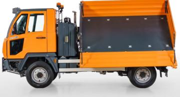
Unloading possible in any direction: large loading area with pendulum tailgate at the rear - ideal for transporting bulk goods or construction site work, for example.
